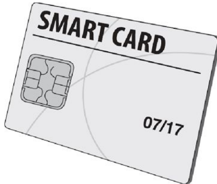
FIGURE 10.1 A smartcard's ISO 7816 interface
