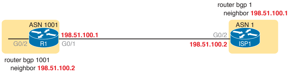
Figure 12-11 Using Link Addresses for BGP Peering in a Single-Homed Design
