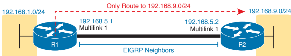
Figure 13-19 Layer 3 Concept Created by Multilink Interface
