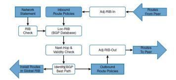
For a specific BGP peer, IOS XE has four options for route filtering, either inbound or outgoing. Each of these approaches can be used independently or in tandem with additional approaches:
