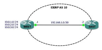
We will filter routes to the three networks connected to router WEST (represented by loopback interfaces) so that they do not show up in the routing table of router EAST. The distribute-list command, a prefix list, an ACL, and a route map will be used to filter each route individually.
