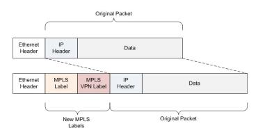
VPN label is for the Egress LSR, so it can identify which traffic belongs to which customer. LDP label is used for the label switching. VPN label is learned from the Provider Edge (PE) router over an MP-IBGP (Multiprotocol Interior Border Gateway Protocol). Label Distribution Protocol (LDP) labels are learned from the Provider Routers in the MPLS domain because they share their label information within the MPLS domain.
