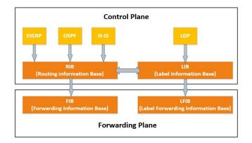
Before enabling MPLS, **Cisco Express Forwarding (CEF)** must be enabled on the routers. In new routers, CEF is enabled by default. It is a technique that makes the switching faster. As discussed above, there is a control plane and a data plane. There is an ARP table in CEF-enabled routers and a routing table in the control plane. Information from the ARP table creates an **Adjacency table** in the data plane, just like a routing table creates a Forwarding Information Base.
