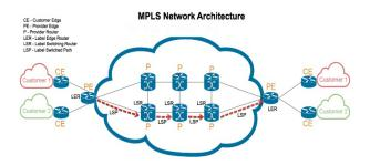
The above figure's red-dashed arrows indicate the Label-Switched Path (LSP). LSP is inside the MPLS domain, where the packet has a label. No label on the packet (unlabeled packet) is not on the LSP and is clearly outside the MPLS domain.
