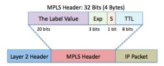
MPLS label header is 32-bit (4-byte) in size and contains four fields. The first 20-bit **Label Value field** has the label value. The next 3-bit **EXP field** is used for Quality-of-Service (QoS). The next 1-bit **S field** tells whether the label is last or not in the stack because there can be multiple labels on a packet (as in VPNs). The last 8-bit **TTL field** has a Time-to-Live value that decreases on every hop till zero.
