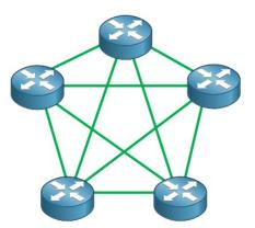
When n = BGP speakers inside the AS, the total number of BGP sessions needed within the AS may be computed using the formula:  $n^{*}(n-1)/2$ . For example, 10 BGP routers would need 45 BGP sessions to have fully meshed.
