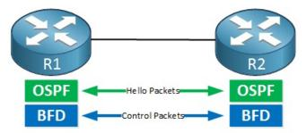
With BFD set up, R1 and R2 will communicate by exchanging control packets. As before, OSPF is still sending its OSPF packets. This will occur once the link fails:
