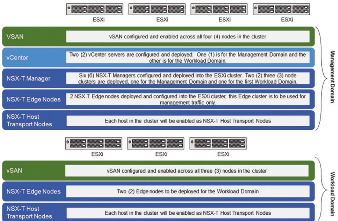
Figure 1-2. Standard Software-Defined Datacenter architecture
