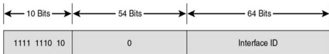
Figure 2-3 IPv6 Link-Local Address Format
