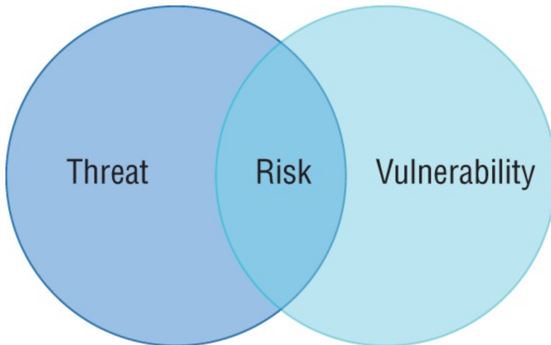
FIGURE 17.1 Risk exists at the intersection of a threat and a corresponding vulnerability.
